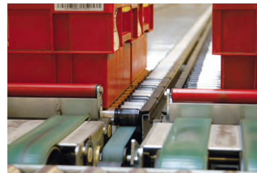
The ORM is friction-driven. The system's rollers, which each have an integral ring, are connected together by a belt
