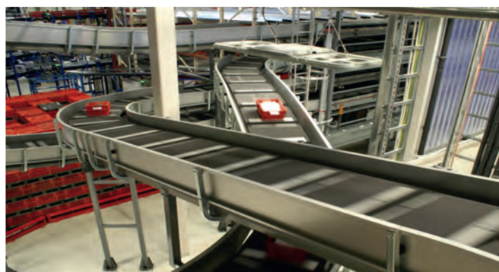
Because of the randomness of Posten Norge's orders, the standard trolley set-up would not offer sufficient capacity, so the company opted for the crates to enter the system via a cross-belt sorter instead
