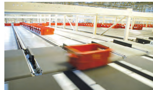
As soon as all the crates for a particular area have been collected, they are released on the output side. The integral dispenser unit ensures that this happens quickly yet in a controlled manner
