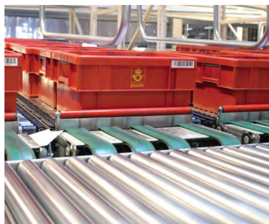
The crates of post travel via the sorter to the ORM on four different levels
