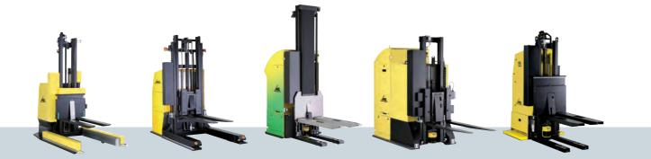
Versions | high-lift fork trucks, straddle trucks, rack stackers, reach trucks, counterbalance stackers, side shift stackers, telescoping fork stackers | Payload | Standard up to 1,500 kg, special up to 4,500 kg | Lift height | 1,200 to 3,000 mm | Safety equipment | Strip sensors, laser scanner with speed-based warning range, soft bumpers | Power supply | Lead, NiCd, Li-Ion, or LiFePo4 batteries
