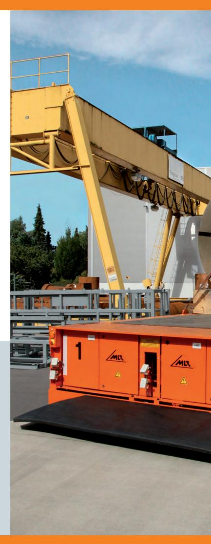
A Caesar P-63.0 Lr transports coils and workpieces in a metal processing plant.
