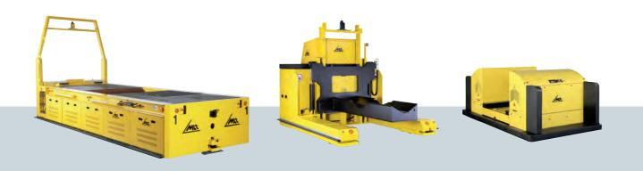
Transport materials | Workpieces, press tools, coils, plates, castings, steel beams | Load capacity | 1.4 to 63.0 tonnes | Vehicle length | Up to 8 meters | Specialized equipment | All-wheel steering, coil fixture | Outdoor vehicles | Radar sensors
